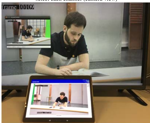
Fig. 14. Playout of hybrid media contents in a Multi-Screen scenario with 3 different views (Linux-based Hybrid Terminal with MS and CS Apps, in PiP mode, and Android-based tablet with CS App)
