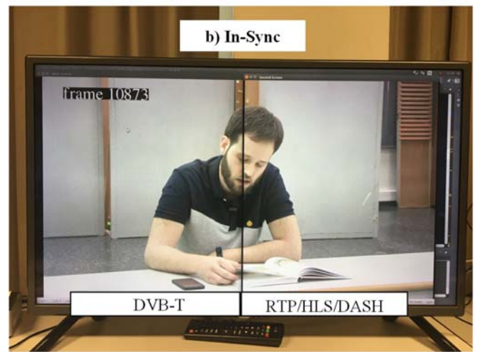
Fig. 18. Video cropping to visually check the sync accuracy
