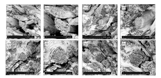
**Figure 9.** SEM images at different magnifications (a, c, e, g taken at  $500 \times$ ; b, d, f, h taken at  $1000 \times$ ) of the fractured surface of fibreboards with PO fibres subjected to different chemical treatments, (**a**,**b**) untreated; (**c**,**d**) NaOH; (**e**,**f**) NaOH + APTMS and (**g**,**h**) NaOH + GLYMO. Black arrows show the improved wetting behaviour between the PO fibres and the surrounding epoxy resin.
