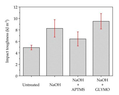
Figure 7. Bar plot of the impact toughness (Charpy test) of PO fibreboards with different surface treatments.
