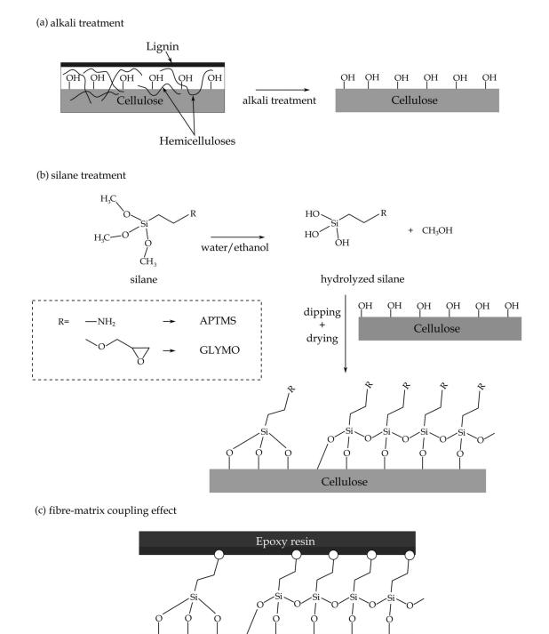
**Scheme 2.** Schematic representation of the effect of alkali and silane treatment on a natural fibre surface and a possible coupling mechanism between PO-treated fibres and epoxy resin.
