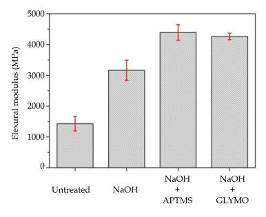
Figure 4. Bar plot of the flexural modulus of PO fibreboards with different surface treatments.
