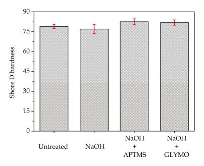
Figure 6. Bar plot of the hardness (Shore D) of PO fibreboards with different surface treatments.
