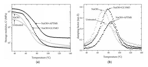
**Figure 8.** Plot evolution of the (**a**) storage modulus (G') and (**b**) damping factor (tan  $\delta$ ) in function of temperature for fibreboards with PO subjected to different surface treatments.
