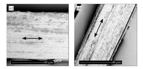
**Figure 5.** SEM images at 1500× longitudinal PO fibres subjected to different chemical treatments, (a) untreated; (b) NaOH; (c) NaOH + APTMS and (d) NaOH + GLYMO (black arrows indicate the fibre axis).
