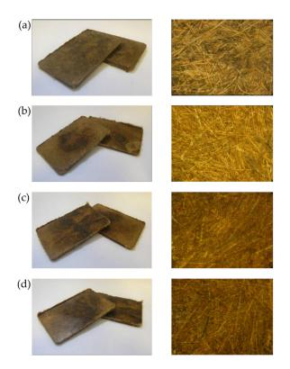
**Figure 2.** Optical images of the fibreboards (**left**) and the surface appearance (**right**) with PO fibres subjected to different chemical treatments, (**a**) untreated; (**b**) NaOH; (**c**) NaOH + APTMS and (**d**) NaOH + GLYMO.
