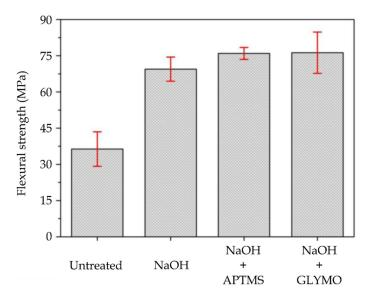
Figure 3. Bar plot of the flexural strength of PO fibreboards with different surface treatments.
