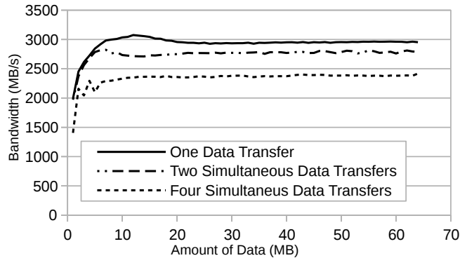
Figure 8: Attained bandwidth when concurrent data transfers to GPUs are performed. Source data is located in the same memory bank.
