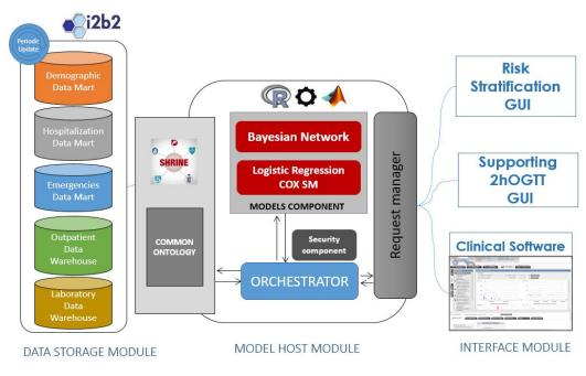
Figure 3. System architecture functional view.
