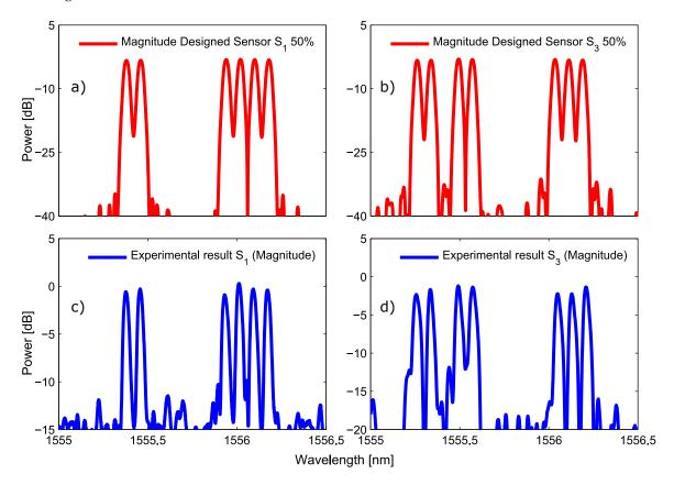
**Figure 8.** The measured magnitude of the manufactured SSFBG is depicted in (c,d) for the devices  $S_1$  and  $S_3$ . The designed magnitude of this sensors is shown in (a,b) for comparison.
