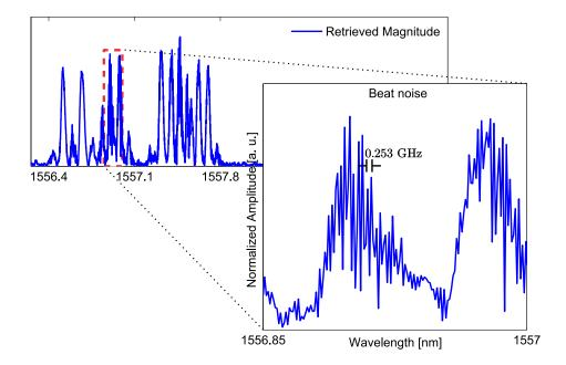
**Figure 5.** Zoomed-in region from a VNA readout. Ripple frequency due to overlapping between two sub-bands is measured to have a frequency of about 0.253 GHz, which is consistent with the placement distance between sensors of approximately 40 cm. (The x-axis represents the scanned wavelength and y-axis represents the normalized amplitude.)
