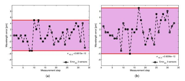
**Figure 10.** Error found for the isolated sensor after comparison with the detected wavelength in presence of a second sensor (**a**), and after comparison with two additional sensors interacting in the same spectral range (**b**).
