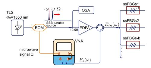
**Figure 3.** Interrogation setup to measure the frequency response of the sensing network. A dual-wavelength scanning source  $E_{in}$  is created by the single side band modulation of a tunable laser at 1550 nm. The reflected waves from the sensing array  $E_s$  are measured at the vectorial network analyzer (VNA) to compute the sensing network frequency response at the fixed microwave frequency  $\Omega$ . OSA: optical spectrum analyzer.
