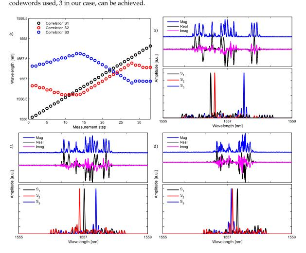
**Figure 9.** Each sensor's central wavelength is depicted for the whole overlapping scenario between the three sensors in (a). (b–d) Three intermediate captures of the system; the upper plot depicts the sensing network readout (magnitude, real and imaginary components) while the lower plot presents the retrieved central wavelength obtained for each sensor after running the correlation algorithm. Magnitude representations have an offset in order to facilitate the visualization.
