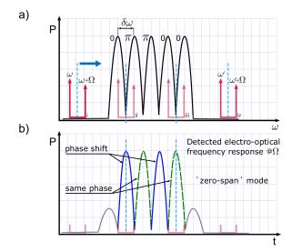
Figure 1. Illustration of the interrogation method used to retrieve the frequency response of the sensing network in phase and amplitude. In (a), the dual-wavelength source scanning process is depicted;(b) depicts the electro-optical frequency response for the sensing device; amplitude and phase response from the sensing array are obtained.
