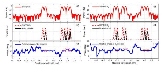
**Figure 7.** Design for the super-structured sensor  $S_1$  and  $S_3$ . (**a**,**d**) Represents the magnitude spectrum in dB for the first and third designed sensor; (**b**,**e**) the linear representation of the magnitude spectrum and their bi-evaluated shape; and (**c**,**f**) the relative phase of the devices  $S_1$ ,  $S_3$ , i.e., the phase relationship between consecutive sub-bands of the device.
