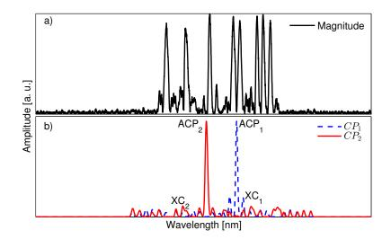
**Figure 4.** (a) Total reflected frequency response of the sensing network composed of two encoded fiber Bragg grating (FBG) sensors; and (b) the correlation product  $CP_k$  computed for each sensor. The corresponding auto-correlation peak (ACP) value points to the matching wavelength location of each sensor in the spectrum. Cross correlation values (XC) are obtained for the remaining wavelength points.
