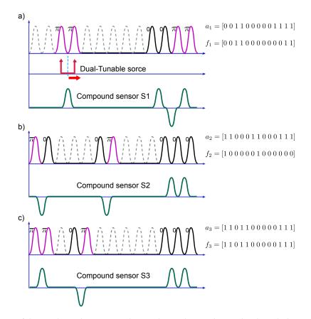
**Figure 2.** Set of three independent sensors designed according to the amplitude and phase codewords reported in Table 1. (**a**–**c**) depict the wavelength sub-band distribution for each super-structured fiber Bragg grating (SSFBG) device as well as their compound signals after interrogation through the dual-wavelength scanning.
