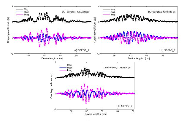
**Figure 6.** Complex coupling coefficient q(z), for the three designed SSFBG sensing devices. The magnitude as well as the real and imaginary components for each sensing device are shown in (**a**–**c**). The amplitude of the coupling coefficient is proportional to the *ac* index profile of the grating.
