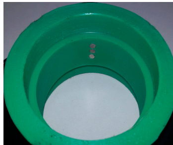
Figure 24. Location of the electrodes in the port.
