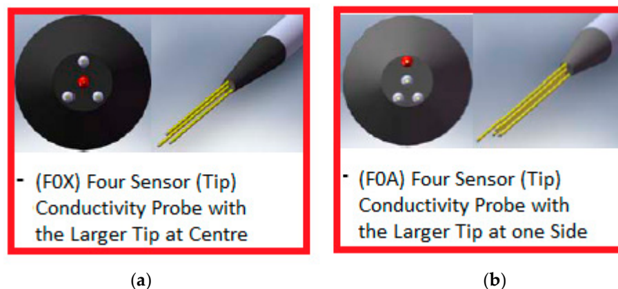
Figure 1. Types of four sensor conductivity probes used to measure the interfacial area concentration, the void fraction distribution and the bubble velocity. (a) Sensor with the larger tip at the center; (b) Sensor with the larger tip at one side
