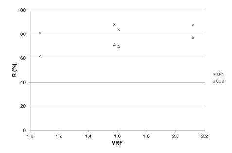
Figure 5. Evolution of T.Ph and COD rejection (R) during the UF as a function of VRF.
