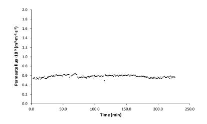
Figure 7. Evolution of the permeate flux in the NF treatment.
