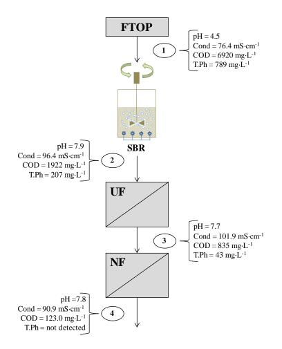
Figure 8. Integrated treatment for the FTOP wastewaters. Streams: (1) FTOP wastewater, (2) SBR effluent, (3) UF permeate, (4) NF permeate.
