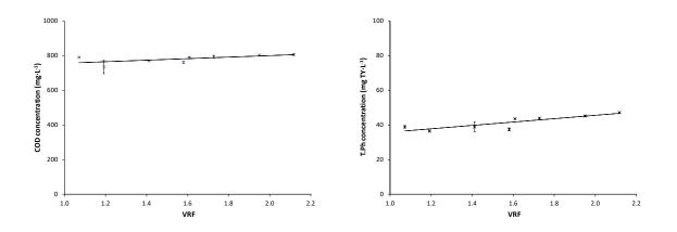
Figure 4. Evolution of the COD and T.Ph concentrations in the UF permeate flux.
