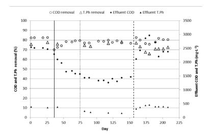
Figure 1. Evolution of the COD and T.Ph removal efficiency and the effluent COD and T.Ph concentration. Vertical lines: [---] FTOP-2; [.....] FTOP-3; [--] FTOP-4.
