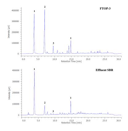
Figure 2. HPLC chromatograms for the effluent SBR and FTOP-3.
