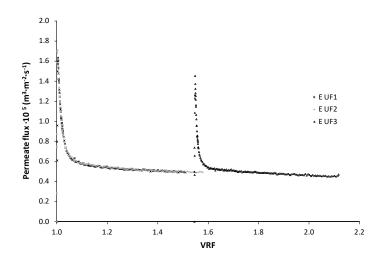
Figura 3. Evolution of the permeate flux with VRF in the UF process for two tests concentrating from a VRF of 1 to 1.57 (UF1 and UF2) and one UF test concentrating with the finals rejections of UF1 and UF2 until reaching a final VRF of 2.10 (UF3).
