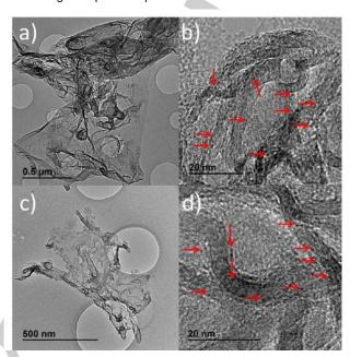
**Figure 4.** TEM images at two different magnifications of  $Ru/NH_2$ -rGO(3.8) before (a and b) and after its use in four consecutive (c and d) reactions. Images (a) and (c) correspond to a general view of the sample before and after reaction, respectively. (b) and (d) corresponds to high-resolution images of (a) and (c) images, respectively, where some Ru NPs have been highlighted with red arrows.
