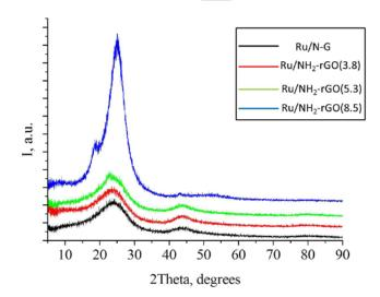
**Figure 1.** XRD patterns of the series of RuCl $_3$  catalysts supported on various modified Gs at 5 % loading. From top to bottom: Ru/N-G (black), Ru/NH $_2$ -rGO (3.8) (red), Ru/NH $_2$ -rGO (5.3) (green), and Ru/NH $_2$ -rGO (8.5) (blue).
