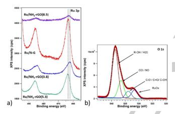
Figure 3. XPS core-level spectra for the  $Ru_{3p}$  region of the Ru/N-containing G samples (a) and best deconvolution XPS core-level spectra for the  $O_{1s}$  region of the  $Ru/NH_2$ -rGO (3.8) sample (b).
