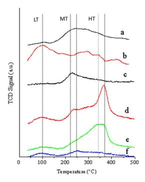
**Figure 5.** CO<sub>2</sub>-TPD profiles of the N-containing Gs without and at 5 wt% Ru loading: a. NH<sub>2</sub>-rGO (3.8); b. NH<sub>2</sub>-rGO (5.3); c. Ru/NH<sub>2</sub>-rGO (3.8) sample; d. Ru/NH<sub>2</sub>-rGO (5.3) sample; e. Ru/NH<sub>2</sub>-rGO (8.5) sample, and f. Ru/N-G sample. Dotted lines correspond to the low temperature (LT), middle temperature (MT) and high temperature (HT) regions.
