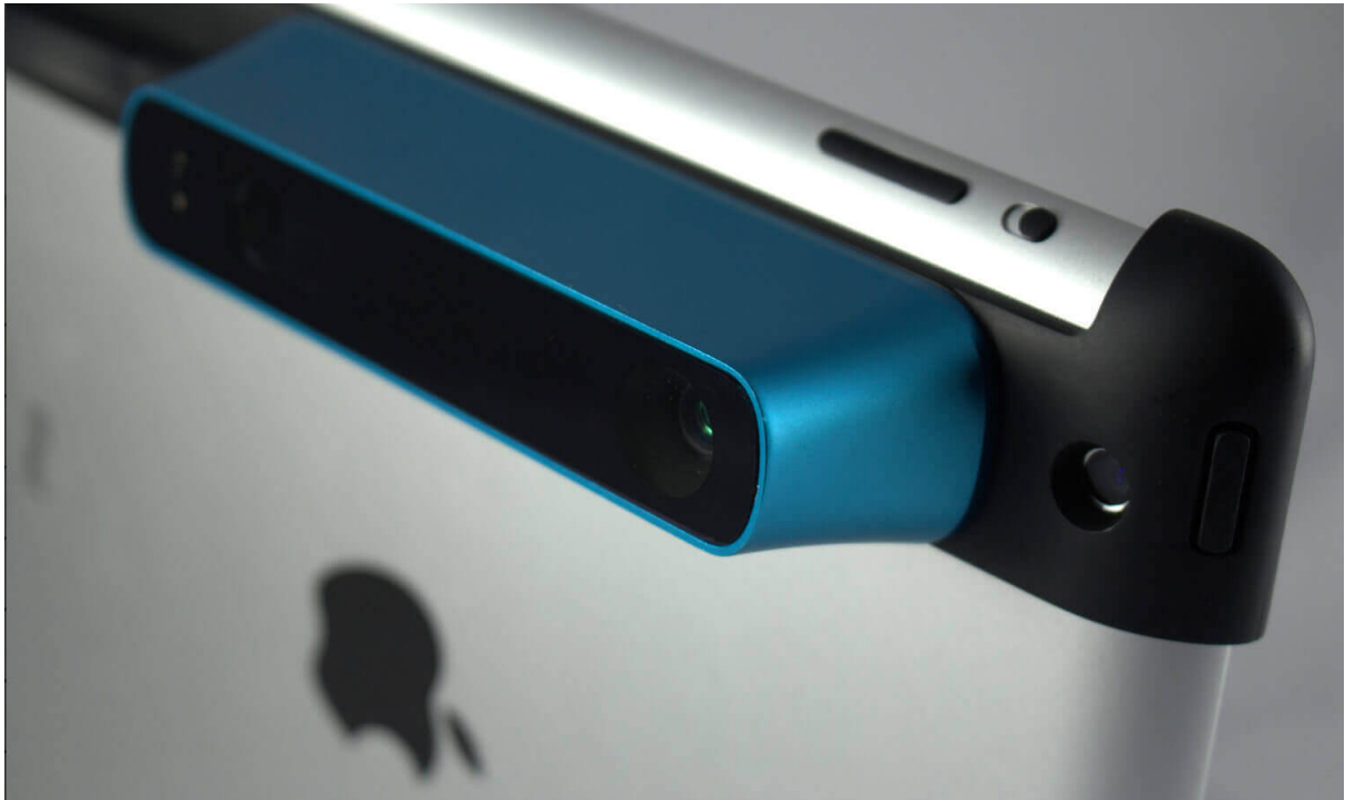
Figura 3. Escáner 3D Structure Sensor
