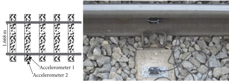
FIGURE 5: Field instrumentation arrangement for the gathering campaign.
