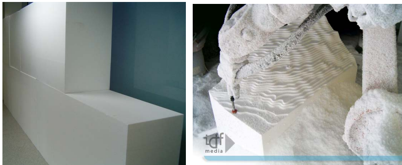
Figure 7.4. Left, EPS blanks; right, machining process of one piece in EPS.
