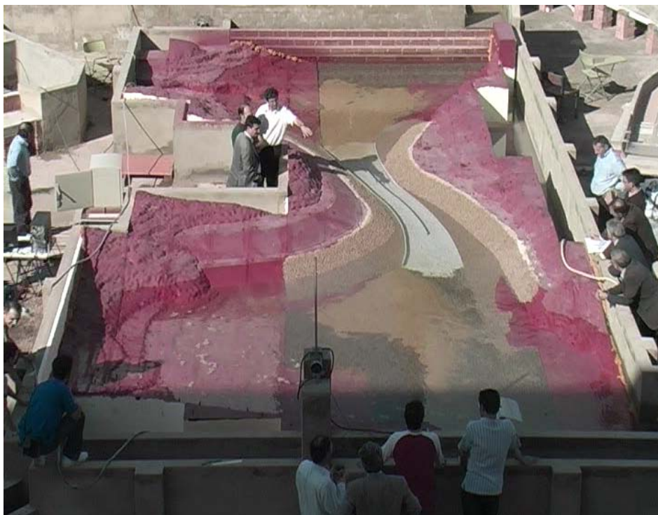
Figure 7.11. Final model in EPS with scaled factor 1:75 for flowing simulation (real dimensions of 8x13 m).
