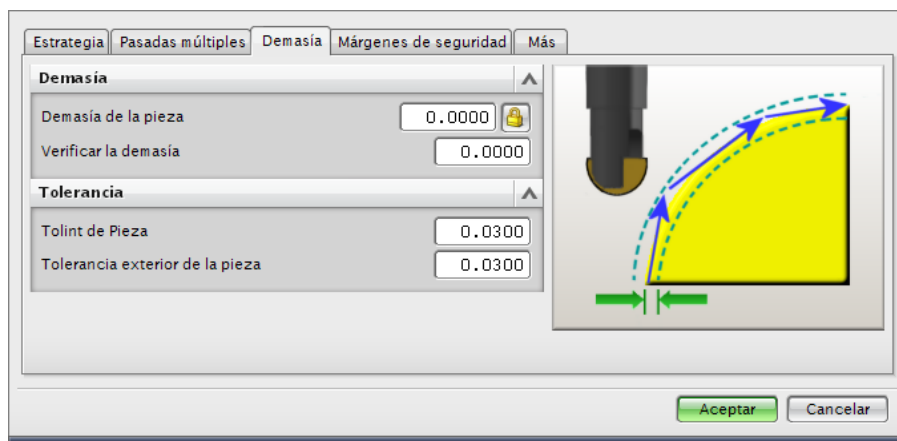
Figure 4.16. Trajectory tolerances, intol and outol , in the NX-CAM system.
