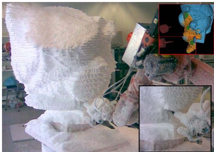
Figure 7.16. The attachment of the blank directly over the table makes the access to the lower parts difficult. Therefore, the blank is fixed by means of an intermediate piece which raises the height.
