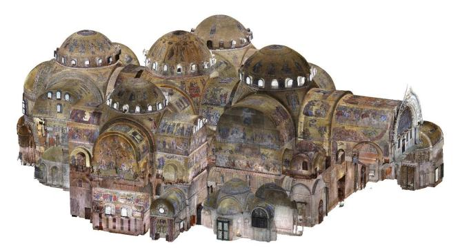
Figure 9: Point cloud of the whole interior space of the Basilica.
