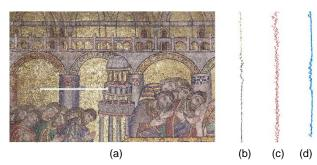
Figure 6: Analysis of the point cloud resulting from the laser scanning survey: comparison between the scanner and the photogrammetric survey: a) detail of the mosaic surface; b) profile extracted from the photogrammetric cloud; c) profile extracted from the Leica C10; and d) profile extracted from the Leica HDS7000.
