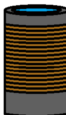
Figure 3. 6 The second solenoid for the first test, which is coiled on a plastic tube that serves as a container
