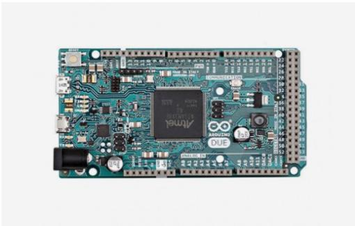
Figura 5.3: Arduino DUE
