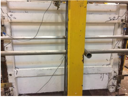
Fig. 8. Failure profile of concrete of specimen T1-NC.
