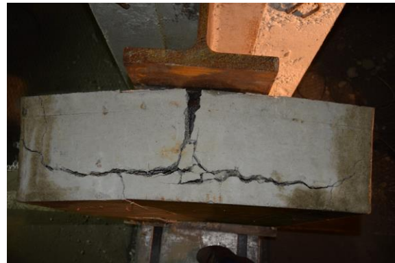
Fig. 8. Transverse bending failure (P22-I).
