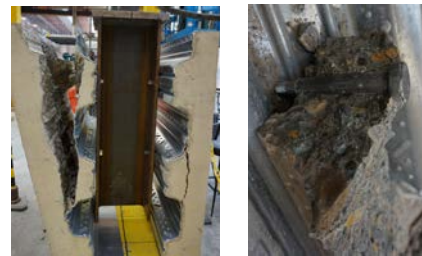
Fig. 7. PUSH-1 after test.
