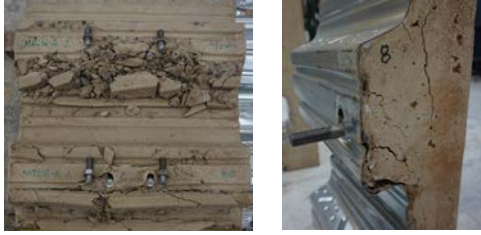
Fig. 11. PUSH-3 after test.
