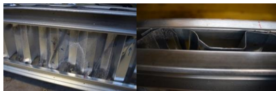
Fig. 15. Distortion of the web corrugation of the CWB SW-1 beam.
