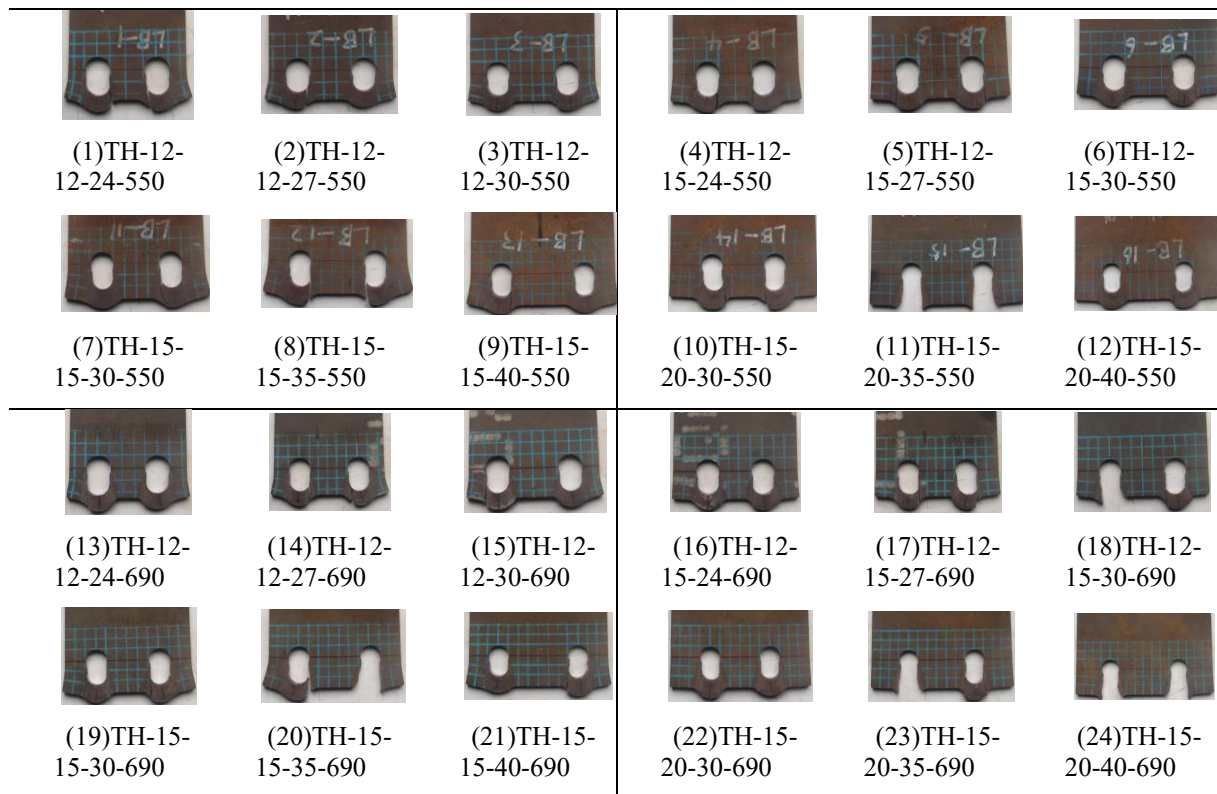
Fig. 4 Failure mode of TH connection
