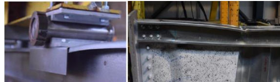
Fig. 18. Local deformations under the load application point.
