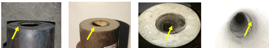
(a) Bamboo sprung back. (b) Buckling of inner steel tube. (c) Crushed concrete.
