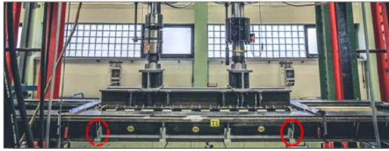
Fig. 19. Global location of failing cracks.
