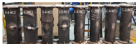
(b) Steel tubes filled with normal concrete.
