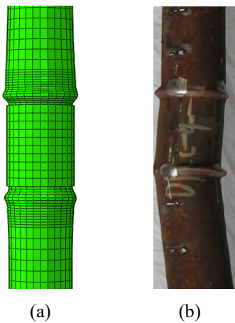
Fig. 1. Final deformed shape of the modelled CFT column under lateral cyclic loading in the (a) FE model, and (b) test [3]
