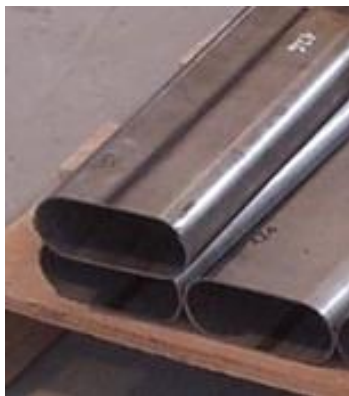
Fig. 2. Round-ended steel tubes.
