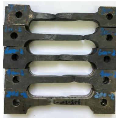
Fig. 8. Failure modes of coupons at elevated temperatures.
