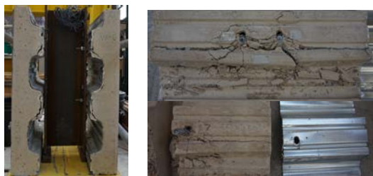
Fig. 9. PUSH-2 after test.
