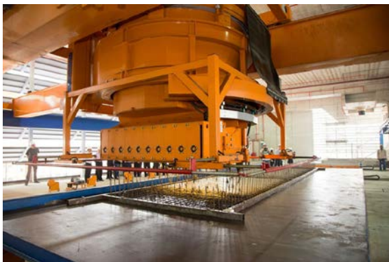
Fig. 13. Highly automated equipment is used in Singapore's Integrated and Prefabrication Hubs to manufacture building components [14].
