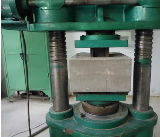
Fig. 1. Test Rigs for Foam concrete specimens test
