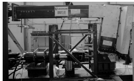
Fig. 25. Beam-column joint after collapse
