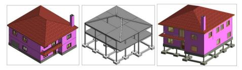
Figure 2: Architectural and structural components of the 3D/BIM model
