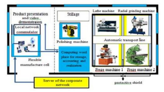
Figure 2. Composes scheme of FMC consisting of mechanical machine tools. Source: Own performance
