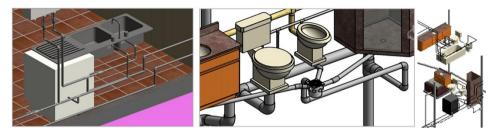
Figure 3: The water supply and the wastewater drainage systems of the BIM model.
