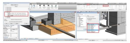
Figure 6: Conflicts between a piping and a bunker structural element
