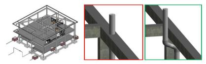
Figure 4: Coordination of structural and MEP disciplines.
