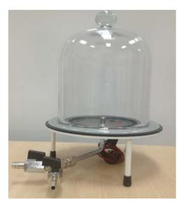
Figure 1. Vacuum pump used to demonstrate the impossibility of sound propagation in vacuum.
