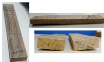
Fig.7: Effect of continuous microwave drying of wood at 300 W of power; Before and after drying.
