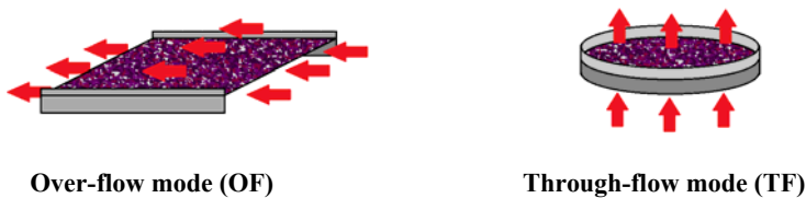
Fig. 1 Hot air direction in two air flow modes inside drying chamber of the dryer.
