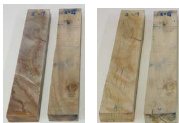
Fig.6: Effect of continuous microwave drying of wood at 500 W; Before and after drying.
