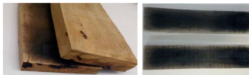
Fig.5: Effect of continuous microwave drying of wood at a maximum power (1000 W).
