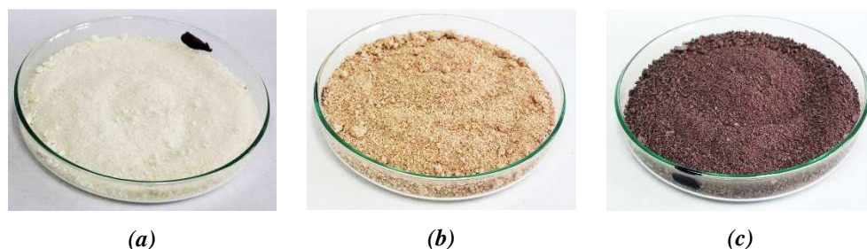
Fig. 1 Dehydrated residues from processing of vegetable milk based on white (a), red (b) and black (c) rice.
