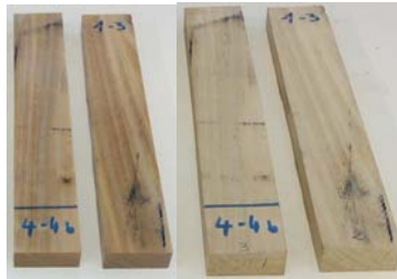
Fig.8: Effect of intermittent microwave drying of wood at 500 W; Before and after drying.
