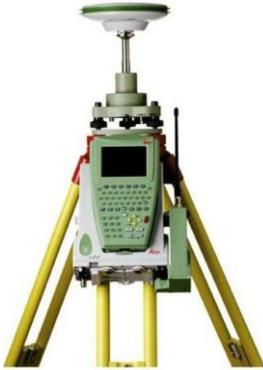
A green and black Leica 1200 GPS Base Receiver mounted on a yellow tripod. The device has a small screen and several buttons on its front panel.                    |
