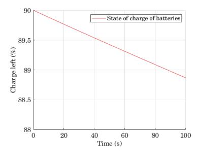
FIGURE 7.4. State of charge variation a levelled flight
