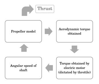
FIGURE 4.6. Flowchart of approximate steps in propulsion block
