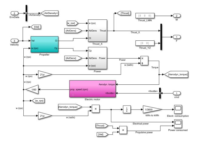
FIGURE 6.1. View of modified propulsion block
