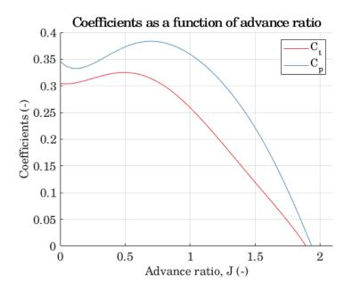
FIGURE 5.9. Polynomial adjustment of the thrust and power coefficients
