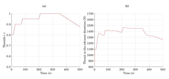
FIGURE 7.6. (a) Throttle variations, ranging from 0.8 to full throttle (b) Thrust variations along the flight
