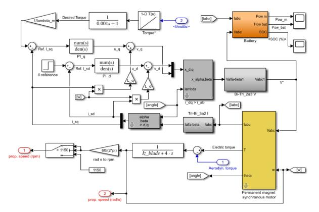
FIGURE 6.5. View of the brushless AC motor in the Simulink environment
