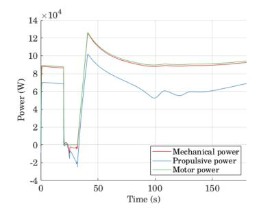
FIGURE 7.14. Power consumption in the case of a simulated motor failure
