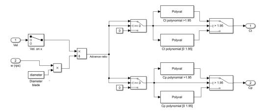
FIGURE 6.2. Propeller subsystem implemented in Simulink
