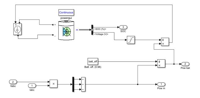
$\ensuremath{\operatorname{Figure}}$  6.7. View of the inside of the battery block
