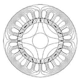
FIGURE 3.4. Halbach magnet array rotor flux distribution (Image from [32])
