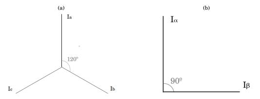
FIGURE 6.4. (a) Triphasic current diagram (b) Biphasic current diagram
