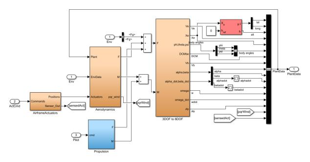
FIGURE 4.4. View of the Vehicle block in asbSkyHogg with the propulsion block in blue
