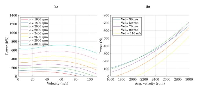
FIGURE 5.5. (a) Power at sea level as a function of velocity, for different angular speeds (b) Power at sea level as a function of angular speed, for different velocities
