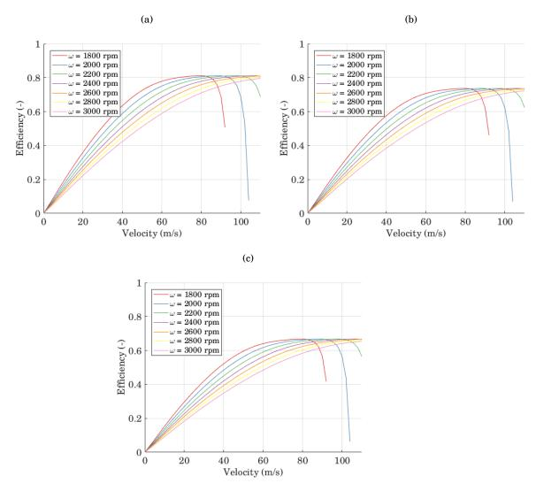
FIGURE 5.7. Efficiency limits for different propeller speeds at (a) sea level (0m) (b) 1000m (c) 2000m
