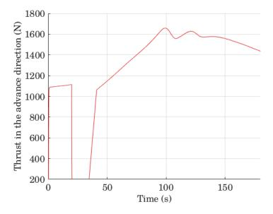
FIGURE 7.15. Thrust as a function of time in a case of motor failure
