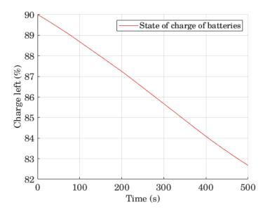
FIGURE 7.10. Battery drainage during the climbs and descents
