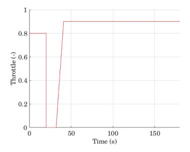
FIGURE 7.12. Throttle commands time in the case of a simulated motor failure
