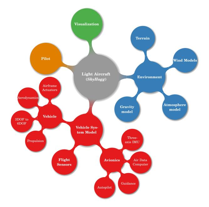
FIGURE 4.1. Diagram of the *asbSkyHogg Simulink* model
