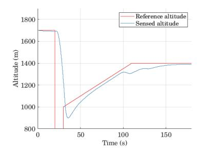
FIGURE 7.11. Altitude against time in the case of a simulated motor failure
