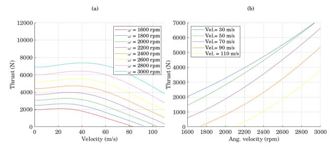
FIGURE 5.4. (a) Thrust at sea level as a function of velocity, for different angular speeds (b) Thrust at sea level as a function of angular speed, for different velocities
