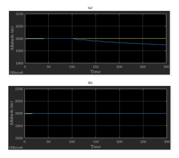
FIGURE 5.1. (a) Case with a thrust of 1300N can not keep levelled flight (b) With 2500N levelled flight can be achieved
