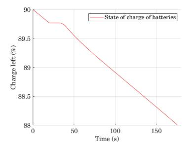
FIGURE 7.16. State of charge variance in a flight with a motor failure
