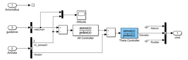
FIGURE 4.3. Default Autopilot block in asbSkyHogg which controls the elevator position
