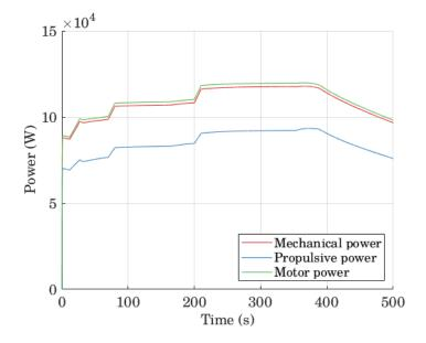
FIGURE 7.8. Power used in different components during the climbs and descents in a flight
