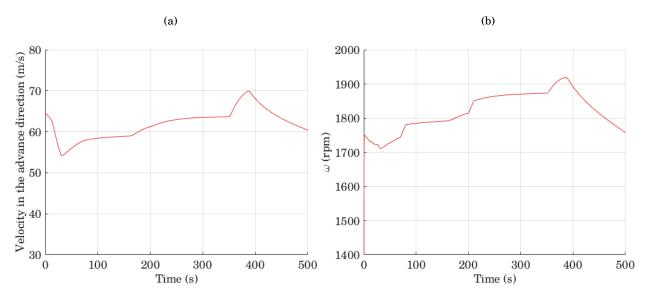
FIGURE 7.7. (a) Velocity in the advance direction variations along the simulation (b) Propeller revolution speed during the simulated flight
