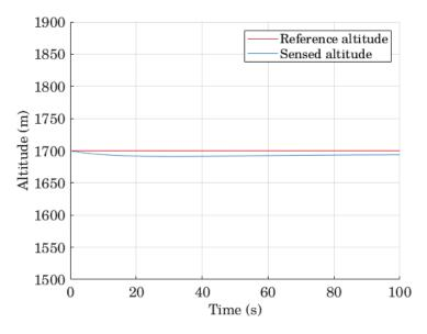
FIGURE 7.1. Vertical profile of a levelled flight at 1700 meters
