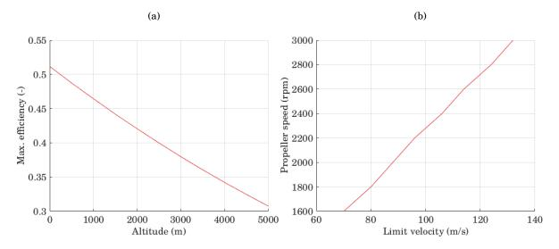
FIGURE 5.8. (a) Maximum achievable efficiency as a function of altitude (0m) (b) Velocity limit for different propeller rotation speeds
