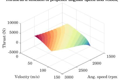
(a) Thrust as a function of propeller angular speed and velocit
