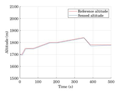
FIGURE 7.5. Vertical profile of the climbs and descents in a flight
