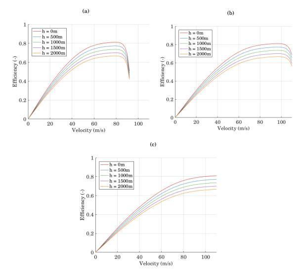
FIGURE 5.6. Efficiency at different altitudes and velocities for a propeller speed of (a) 1800rpm (b) 2200rpm (c) 2600rpm
