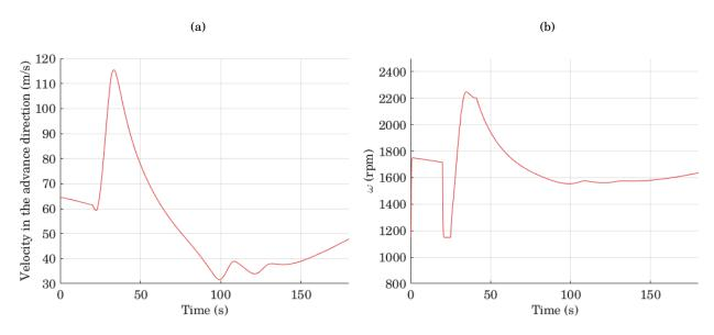
FIGURE 7.13. (a) Velocity in the advance direction variations along the simulation (b) Propeller revolution speed during the event
