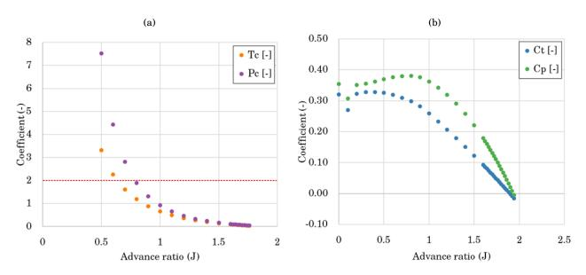
FIGURE 5.2. (a) Traditional thrust and power coefficients used in aeronautics (b) Thrust and power coefficients defined by *JavaProp* as propeller coefficients
