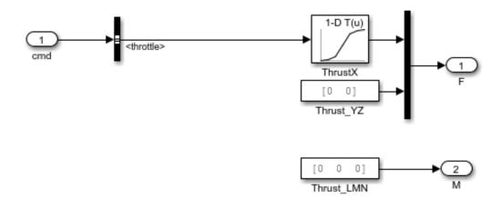
FIGURE 4.5. Default propulsion block in asbSkyHogg
