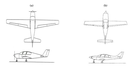
FIGURE 6.6. Comparison between similar aircrafts (a) The *SkyHogg* plans (b) Plans of the *Lancair IV* [53]
