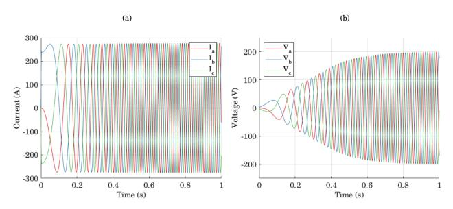
FIGURE 7.3. (a) Triphasic current levels for the first second of levelled flight (b) Triphasic voltage levels for the first second of levelled flight
