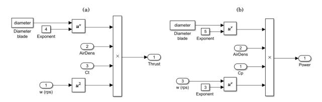
FIGURE 6.3. (a) Thrust subsystem in Simulink (b) Power subsystem in Simulink
