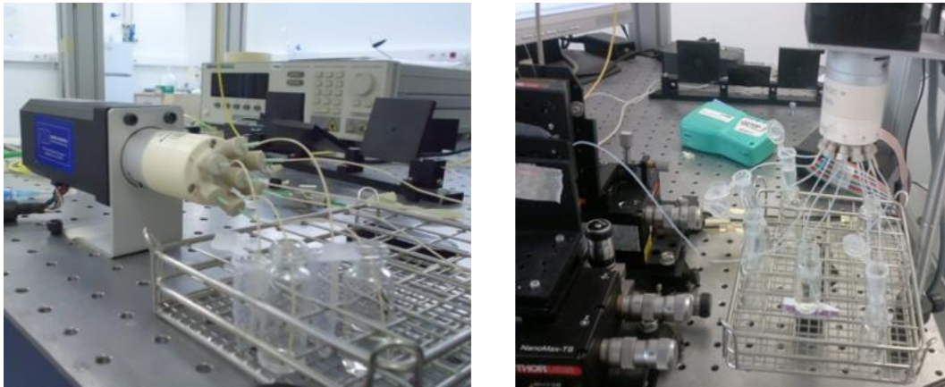
Fig. 2.16: Pictures of the automatic fluidic switch.
