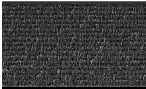
Fig. 3.20: SEM cross-sectional image of the fabricated PS multilayer structure.
