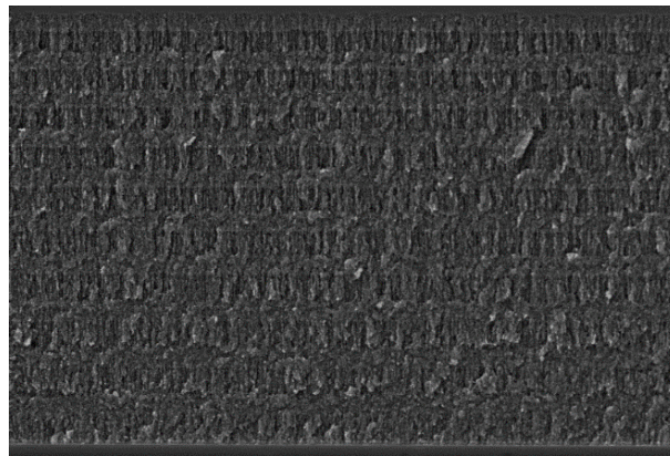
Fig. 3.25: SEM cross-sectional image of the second fabricated Bragg reflector.
