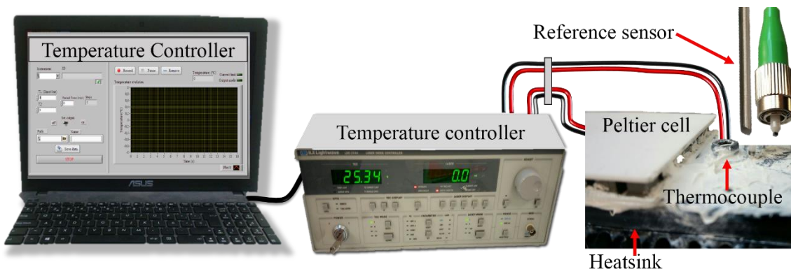
Fig. 4.5: Illustration of the thermal setup.
