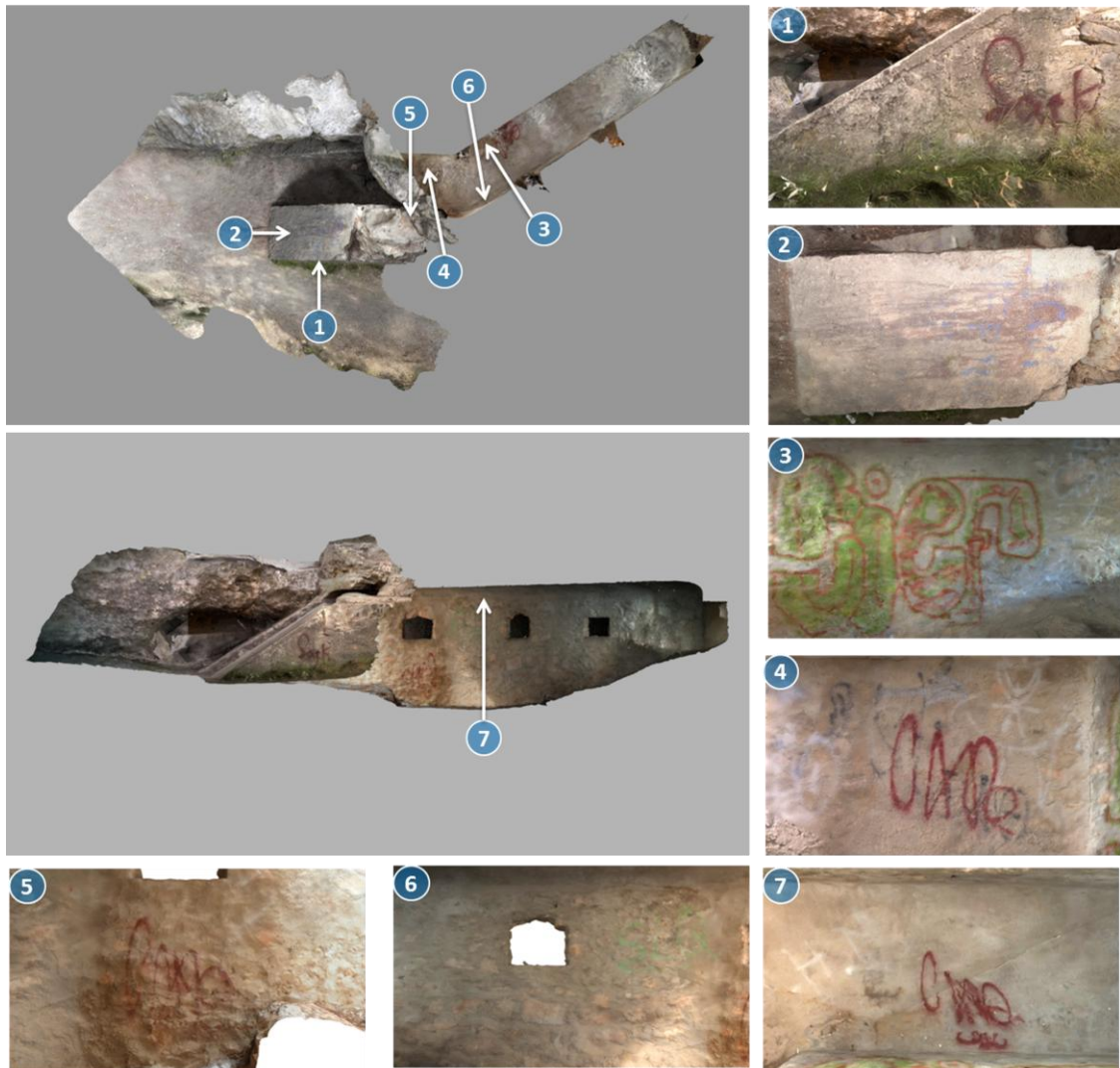
265 Fig. 7. Camera settings. Location and view angle are adjusted to cover the seven areas of interest (1 to 7).
