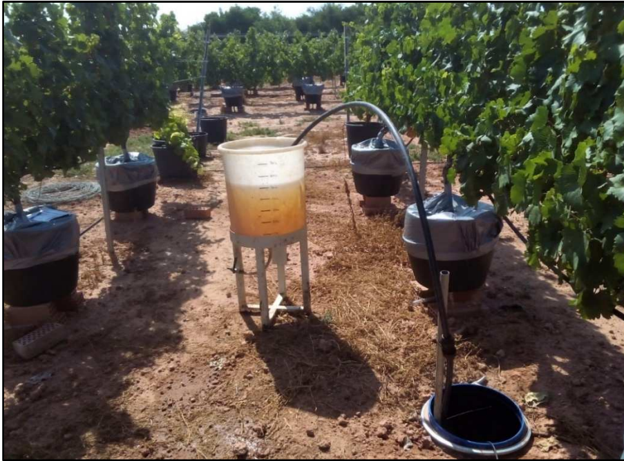
Figure 19. Emptying and measuring the water volume of the underground drainage collector system, which included a reservoir per each five vines during seasons 2015 and 2016.
