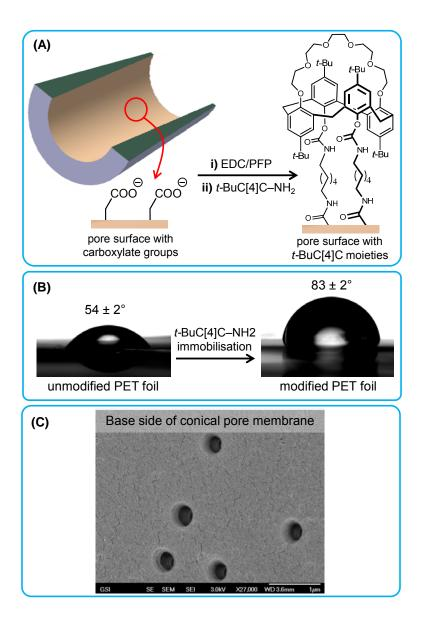
**Figure 3.** (A) The functionalization of the carboxylic acid groups on the surface of asymmetric nanopore with *tert*-butylcalix[4]arene–crown (t-BuC[4]C) moieties via carbodiimide coupling chemistry. (B) The contact angles of an unmodified PET membrane with carboxylic acid groups and a functionalized membrane having t-BuC[4]C moieties. (C) FESEM image of the base opening side of the conical pores in a PET membrane having  $10^7$  pores cm<sup>-2</sup>.
