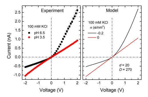
**Figure 2.** Experimental and theoretical I-V characteristics of the as-prepared single conical pore recorded in 100 mM KCl solution at pH 6.5 and 3.5, separately.
