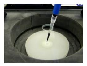
Figure 5.1. Spin-coating process (feeding of dissolved metal solution onto ITO substrate using micropipette).
