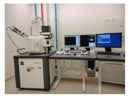
Figure 3.7. image of scanning electron microscopy (FE-SEM), a Zeiss ULTRA 55
