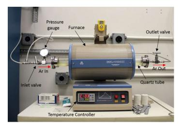
Figure 3.2. The sulfurization/selenization setup.
