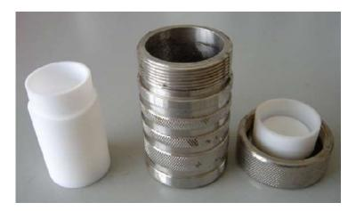
Figure 3.3. A typical Morey autoclaves.
