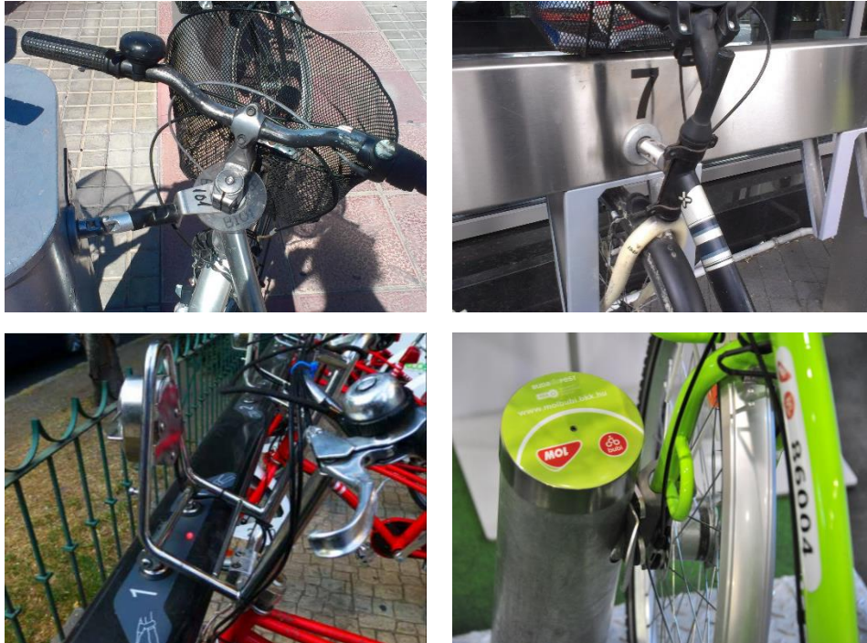
Figure 8: Examples for docking mechanisms Top left: bicielx, Elche, Top right: Rentbike Hotel by MOVUS, Valencia Bottom left: Ecobici, Buenos Aires (Source: ITDP - The bikeshare planning guide 41 ) Bottom right: MOL Bubi, Budapest (Source: BKK 42 )
