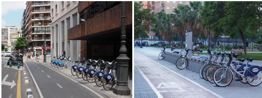
Figure 41: Good practice: Valenbisi station placement The bicycles are directly accessible from the bike-path. However, it would be better if the bikes on the right were placed in the opposite direction.
