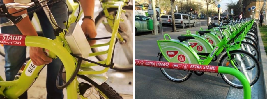
Figure 28: MOL Bubi’s extra electronic lock and bike stand Left - Bike secured to the extra bike stand (Source: Mol Bubi Google+ 126 ) Right - Docking station with the extra stand (Source: autoszektor.hu 127 )
