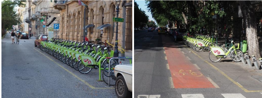
Figure 32: Good practices - MOL Bubi stations in the parking lane with direct access to road surface and cycle lane. This design eliminates the conflicts between pedestrians and cyclists while provides more space for sustainable urban mobility by reclaiming former car parking spots for cycling.
