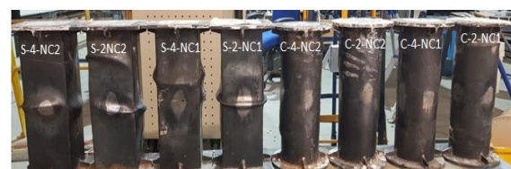
(b) Steel tubes filled with normal concrete.
