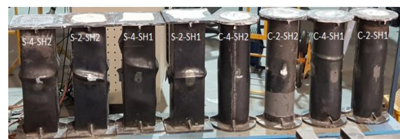
(a) Steel tubes filled with SHCC.
