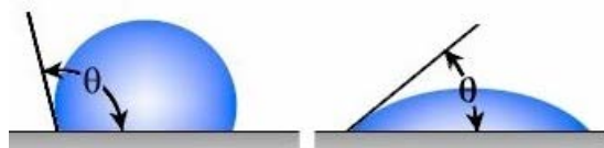
Figure 2.24. Contact angle measurement for hydrophobic (left) and hydrophilic (right) surfaces.
