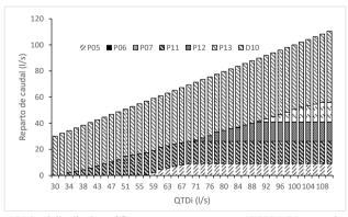
Fig.5. Optimal distribution of flows among water sources. COPLACA network
