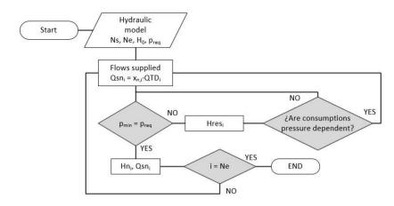
Fig. 1. Process to get setpoint curve (SC)
