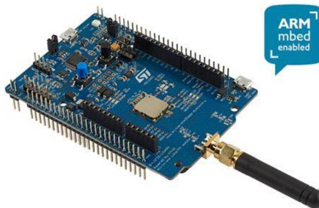
Figura 36 - B-L072Z-LRWAN1 - STM32L0 Discovery kit LoRa
