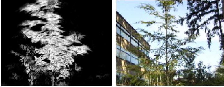
Figure 6.6: On the left, image showing the areas in which background models were changed in order to adapt to changes in the background. The frame corresponds to an outdoor sequence of the Wallflower benchmark. On the right, one frame of the original sequence.
