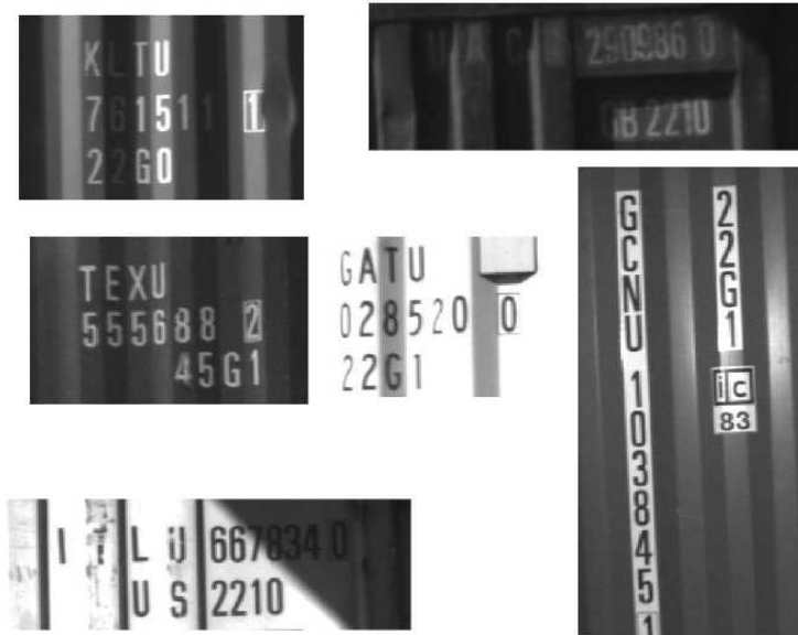
Figure 4.2: Some sample images representing truck containers. As explained in the text, note the wide variability of possible situations, that the designed algorithm has to face.
