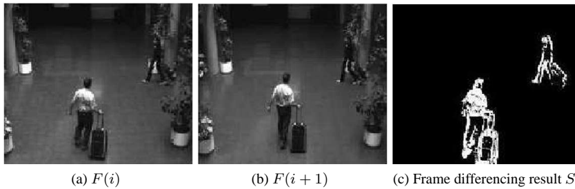
Figure 3.4: Example of frame differencing. Figure 3.4a and 3.4b are subtracted and the result is shown on Figure 3.4c, note that only pixels which are very close to the border of the objects are marked as foreground.
