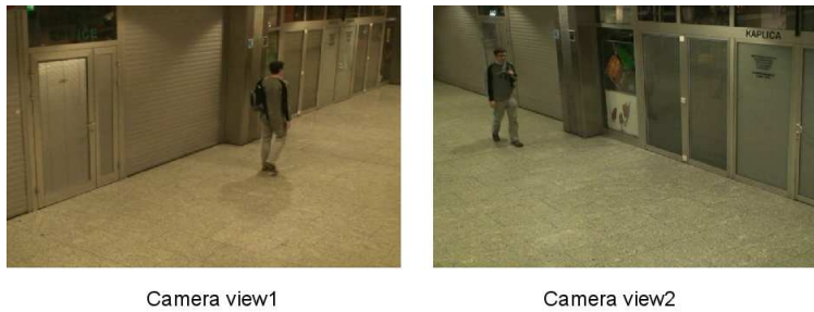
Figure 5.2: Two different cameras whose fields of view overlap. Note that the person in the field of view of camera 1 is also seen by camera 2.
