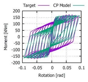
*Fig.* 7. Lateral load versus rotation comparison between the target data and the calibration results
