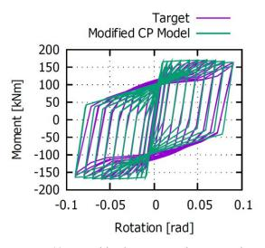
*Fig. 10.* Lateral load versus rotation comparison between the target data and the calibration results of the modified CP model
