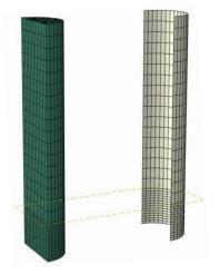
Fig. 2. Geometry of the 3D FE model
