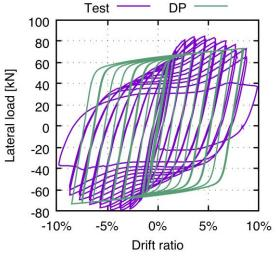
Fig. 5. Lateral load versus drift ratio comparison between test results and DP model prediction
