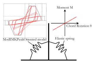
*Fig. 8.* The modified CP model proposed for a CFST member
