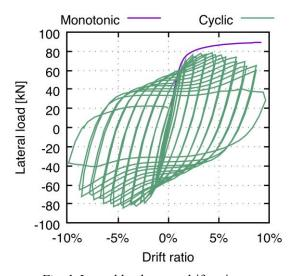
Fig. 1. Lateral load versus drift ratio curves -Comparison between specimens under monotonic and cyclic loading
