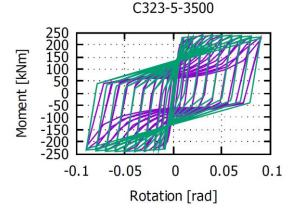
*Fig. 11.* Comparison between the ABAQUS cyclic response and the calibration results of the modified CP model
