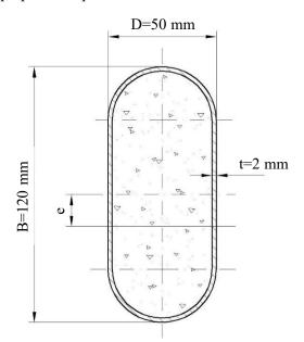
Fig. 1. CFRT column cross-section.
