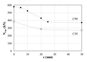
Fig. 3. Experimental ultimate load vs eccentricity.
