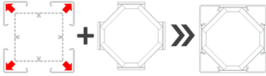
Fig. 2. Basic concept of composite mega column
