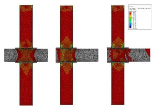
b) Lateral c) Corner Fig. 7. Lateral stress S11, at strains of 0.005.
