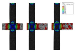
a)Central b) Lateral c) Corner Fig. 6. Vertical stress S33, at strains of 0.01.
