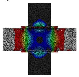
Fig. 11. Natural arch effect between the plates.
