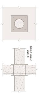
Fig. 1. Slab-column connections without continuity of the tube.
