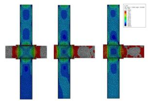
a) Central b) Lateral c) Corner Fig. 5. Vertical stress S33, at strains of 0.005.
