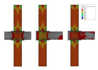
a) Central b) Lateral c) Corner Fig. 8. Lateral stress S11, at strains of 0.01.
