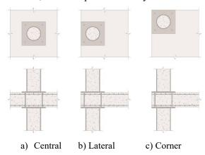
Fig. 3. Slab-column connections without continuity of the tube.
