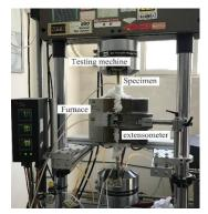
Fig. 6. Test setup at elevated temperatures.
