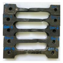
*Fig. 8.* Failure modes of coupons at elevated temperatures.
