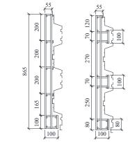
Fig. 3. Design of reinforcement cages (side view).
