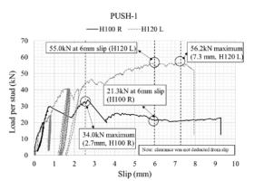
Fig. 6. Comparison of load vs. slip curves (PUSH-1).
