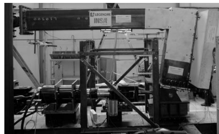
Fig. 25. Beam-column joint after collapse
