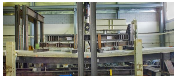
Fig. 12. Deflection of the beam after test
