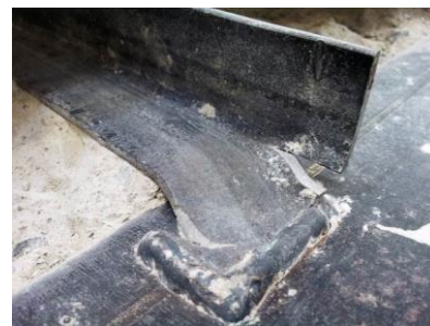
Fig. 7. Angle deformations after testing
