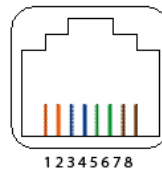
Fig. 4: “Conector P/T CONTROL IN SERIAL (RJ-45)”
