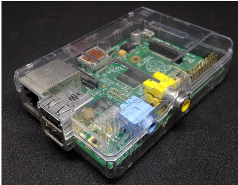
**Figura 4.2:** Raspberry Pi modelo B.
