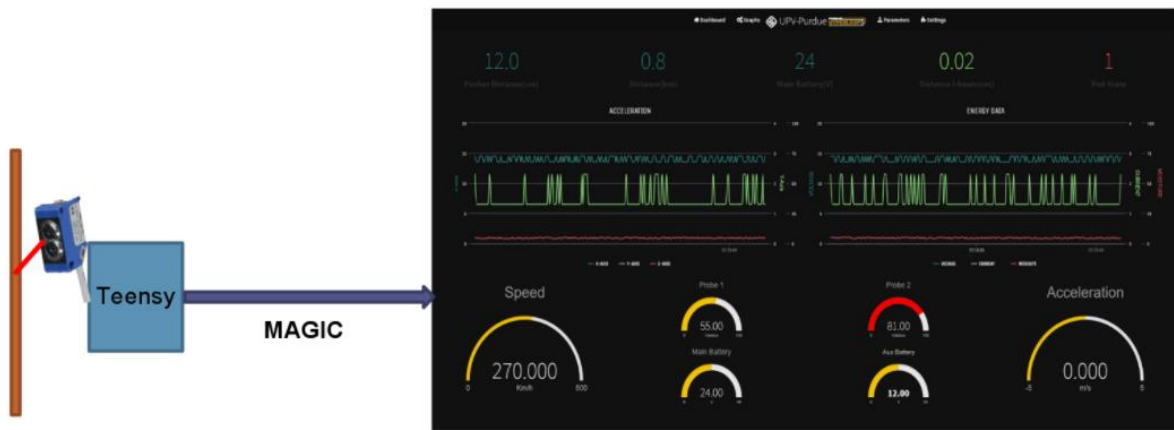
Figure 50 Schematic of the Avionics system showing the GUI and the connection with the sensor and microcontroller (Vicén 2017).
