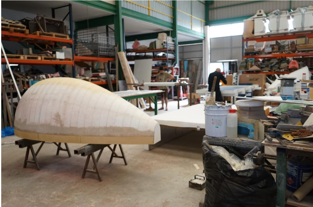
Figure 55 At the workshop in Beniflà, preparing the fairing mold (Vicén 2017).
