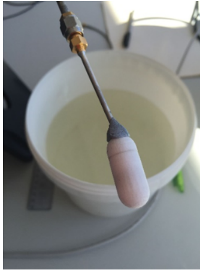
Figure 3.31: Discone antenna embedded into a polyethylene capsule.
