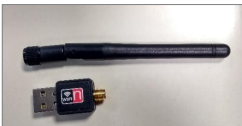
Figura 7. Antena Raspberry Pi Ralink Chip Rt5370.
