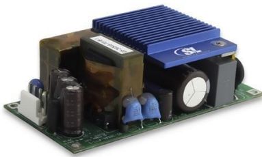
Figura 15. Transformador AC-DC Condor / SL Power MB120S15K01.
