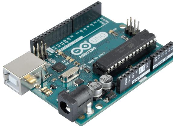
Figura 2.9: Hardware Arduino UNO
