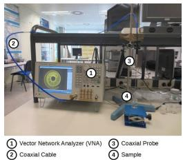
Fig. 1. Setup of the coaxial probe connected to the vector network analyzer.
