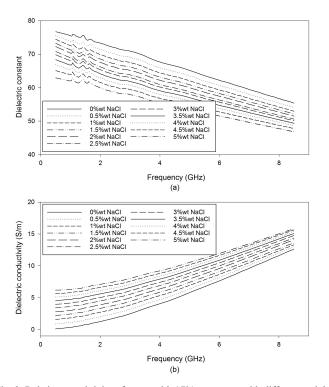
Fig. 3. Relative permittivity of water with 17%wt sucrose with different weight concentrations of NaCl: a) Dielectric constant b) Dielectric conductivity.
