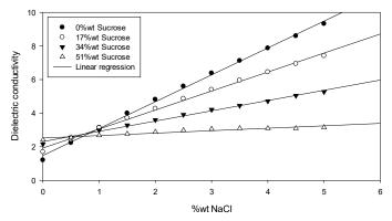
Fig. 8. Influence of sodium chloride on dielectric conductivity at 2.4 GHz in aqueous solutions of sucrose.
