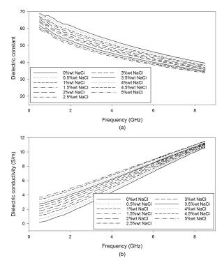
Fig. 4. Relative permittivity of water with 34%wt sucrose with different weight concentrations of NaCl: a) Dielectric constant b) Dielectric conductivity.
