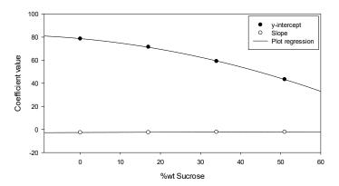
Fig. 7. Y-intercept and slope of series shown in Fig. 6 with respect to sucrose concentration.
