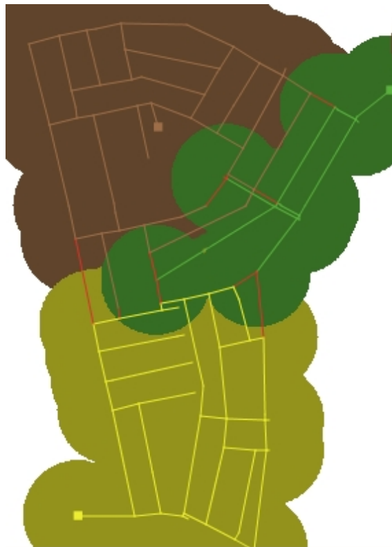
Figure 7. Final distribution of hydraulic sectors
