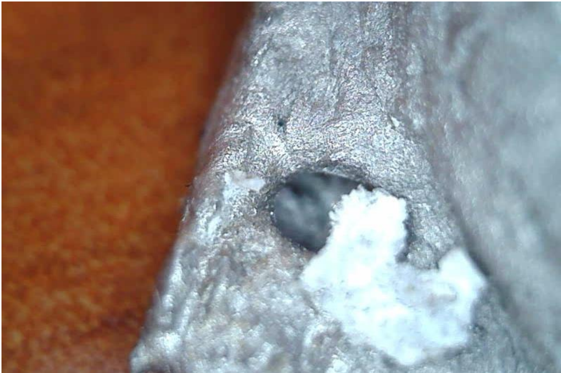
Figure 26: Casted part, occurring holes
