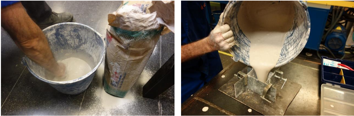
Figure 11: Mixing and pouring of the gypsum
