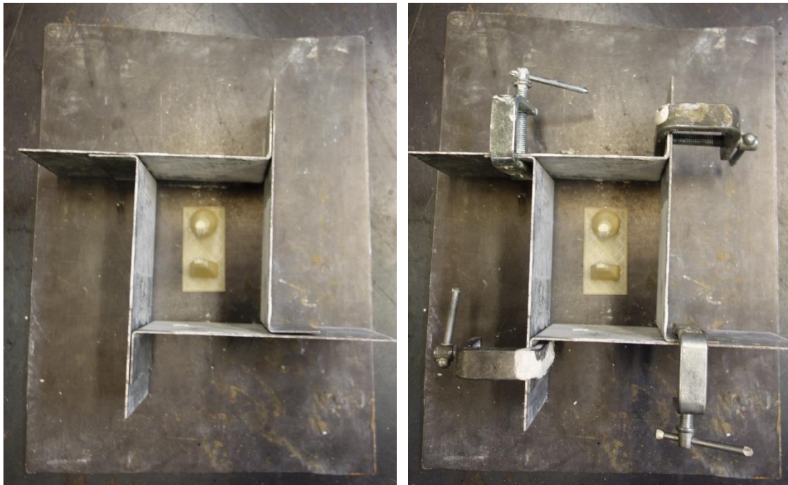
Figure 9: Arranging the mould
