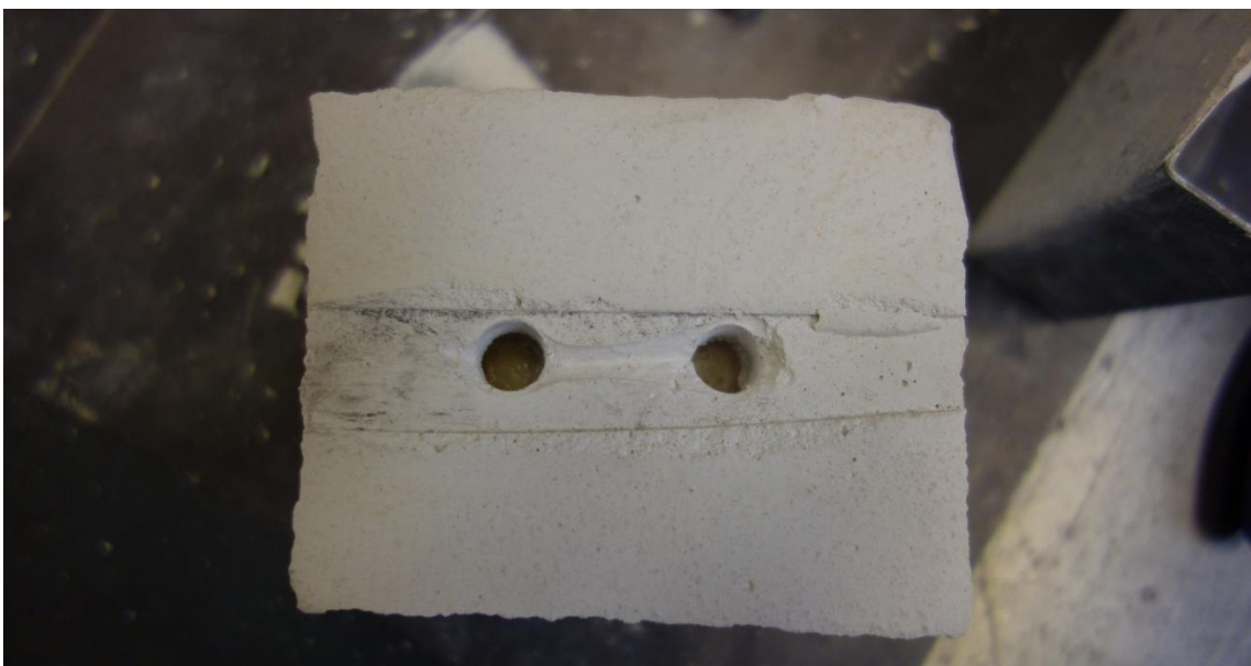
Figure 14: Mould without the helping structure
