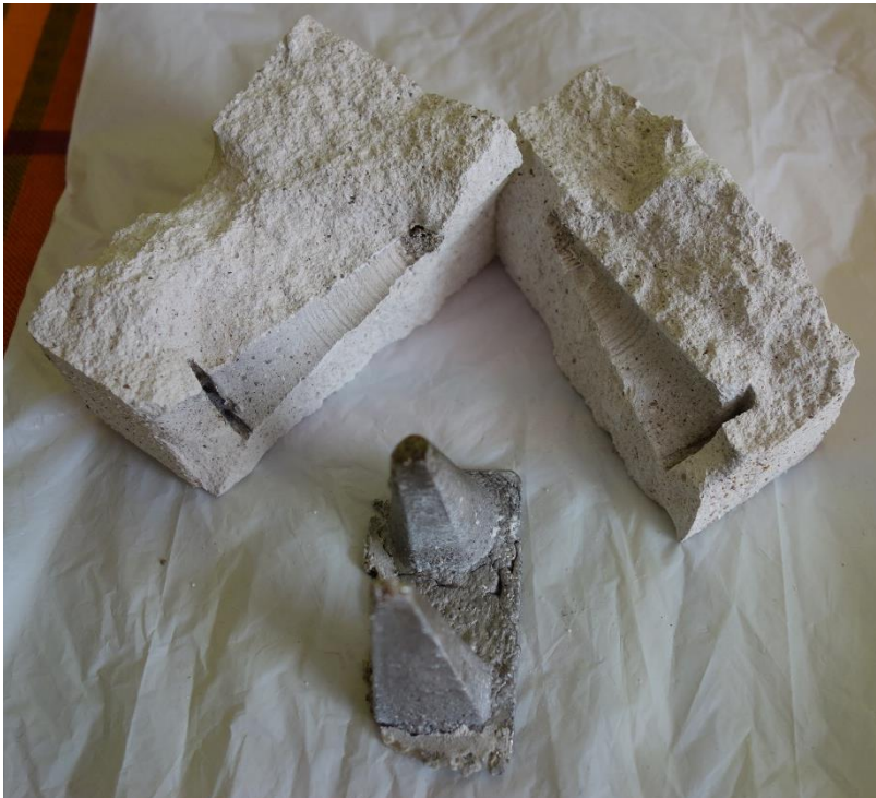
Figure 30: Mould and casted part
