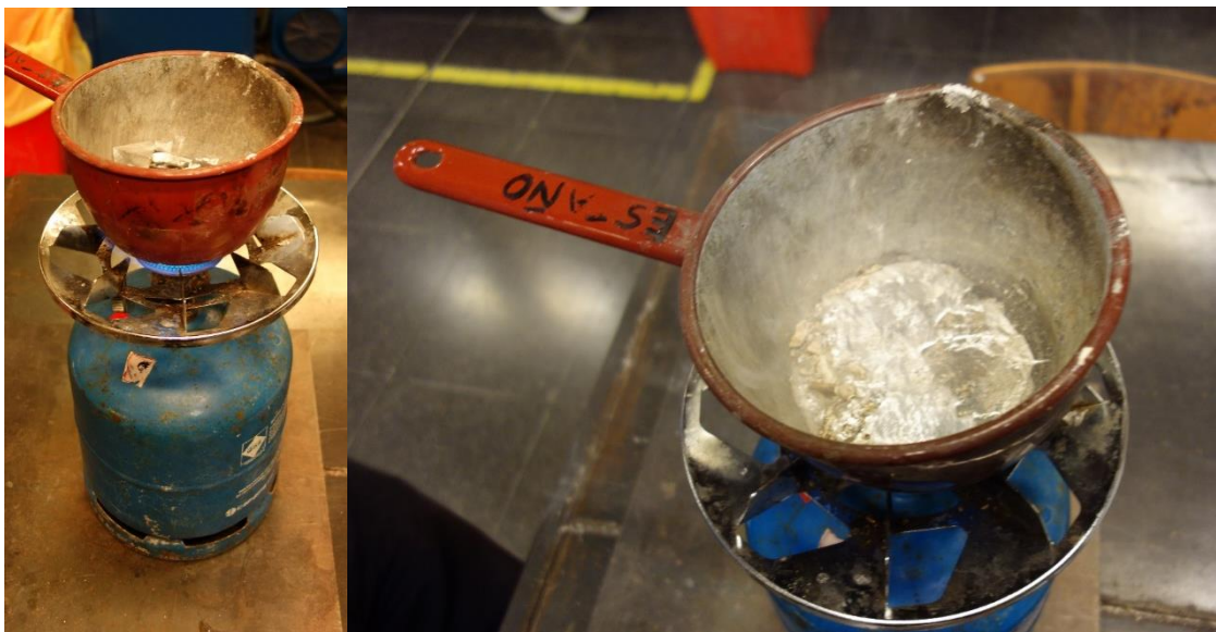
Figure 18: Melting the lead
