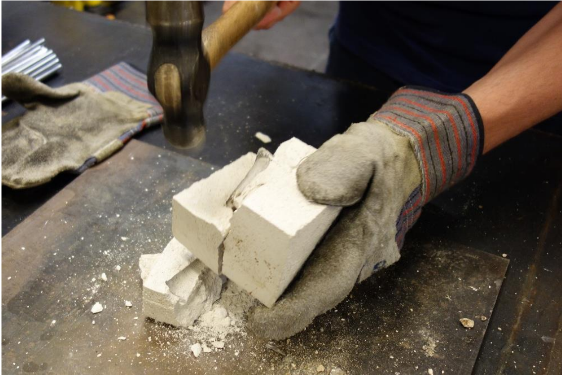
Figure 21: Removing of the mould with a hammer
