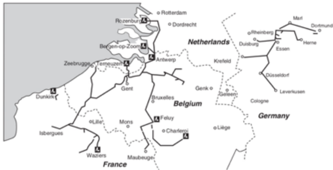
Fig. 11.2 Hydrogen pipeline network in north-western Europe – Roads2HyCom (2007)
