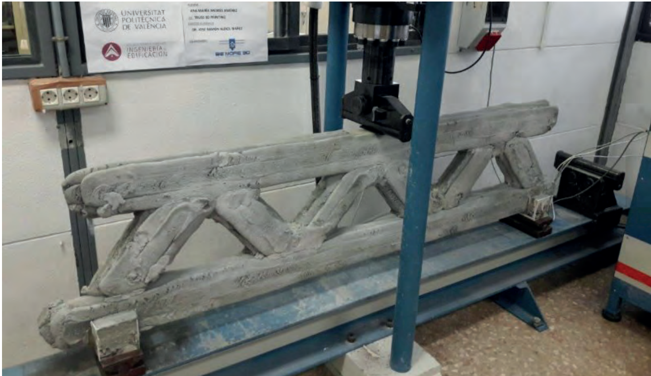
Figura 5. Imagen prototipo cercha impresa. BEMORE3D (2017) / Figure 5. Image of printed truss. BEMORE3D (2017).
