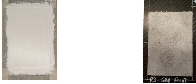
Figure 5.25: Sample preparation with white coat and graphite spray.
