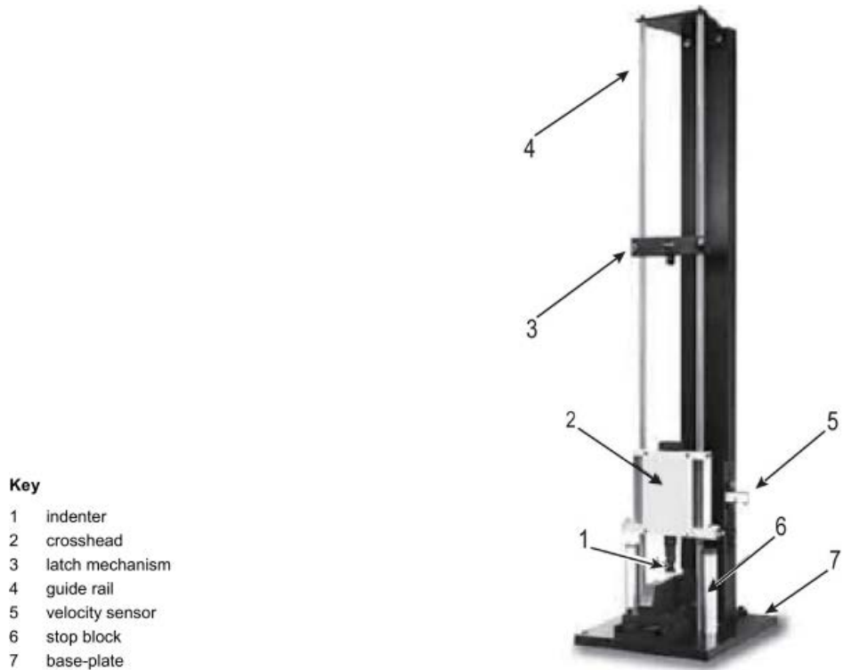
Figure 2.3: Instrumented drop-weight impact device with double guide rails [11].
