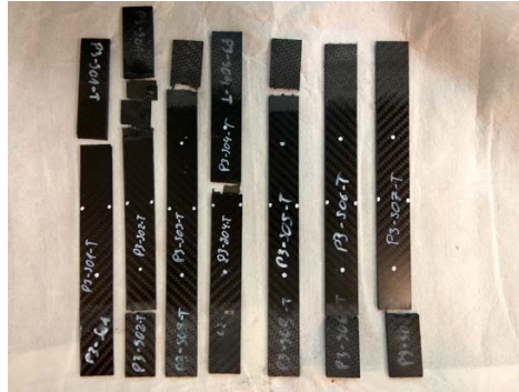
Figure 4.6: Tensile test samples failure.
