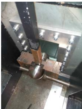
Figure 5.3: Pictures of the pendulum masses, indenter and sample clamp frame.
