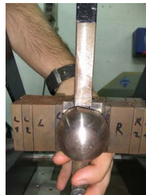
Figure 5.3: Pictures of the pendulum masses, indenter and sample clamp frame.
