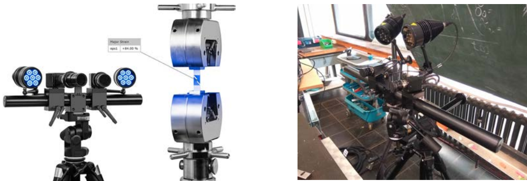
Figure 5.24: ARAMIS adjustable – 3D Motion and Deformation Sensor.
