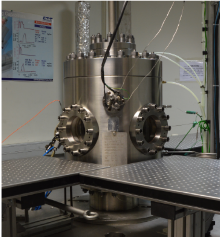
Fig. 4.7 High temperature and high pressure test rig
